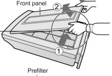
3 Remove the pre-filter, and then remove the stamina-power carbon (black) and HEPA filter (white) that are inside the polyvinyl bags.
